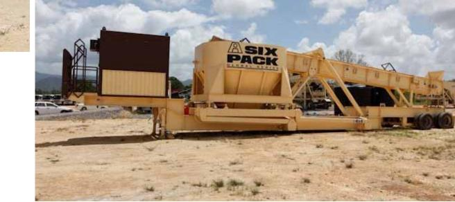
lagged head pulley, self-cleaning tail pulley and 5 HP variable speed drive, 3'x 6' single deck scalping screen, 24" inclined conveyor with 5 HP drive, gravity take-up, belt scale, load cells, and drum bypass. Package is all mounted on a single axle frame. A cable tray is provided along one side of the frame for routing of cables.
