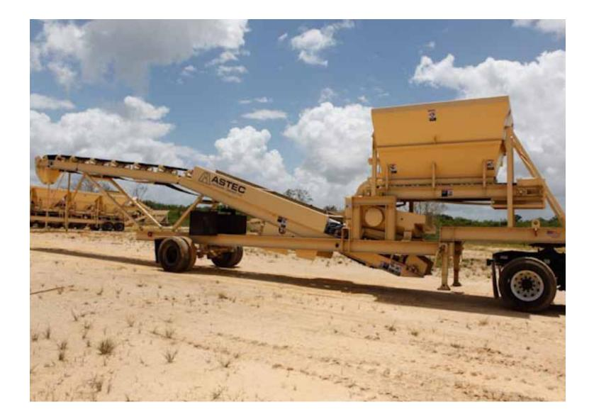
built-in sampling ports that are easily accessible. Portability is provided on a fully equipped tandem axle frame with air brakes, signal lights, spring suspension, kingpin, and glad hands. It also has telescoping support legs that are adjustable. A cable tray is provided along one side of the frame for routing of cables.
